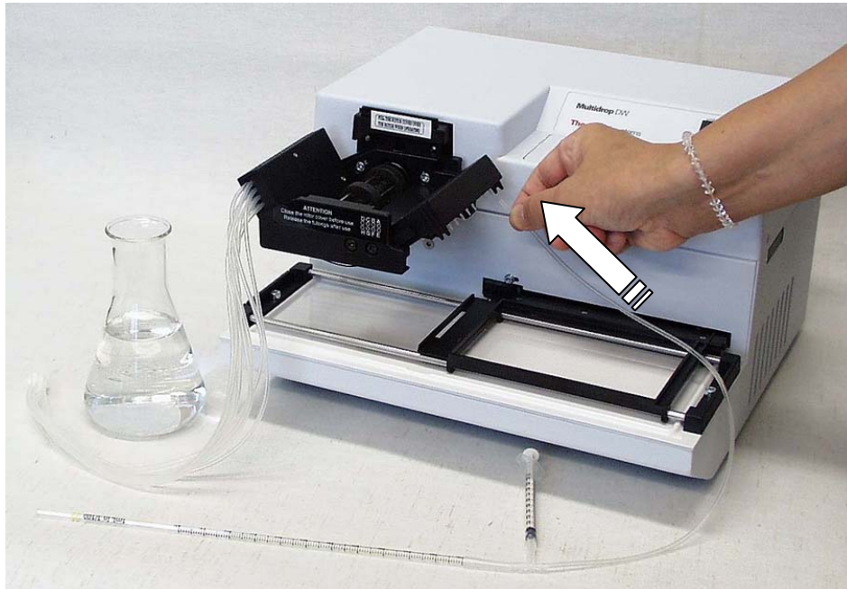
Fig. 7.5 Placing the tube onto the tip of channel A
