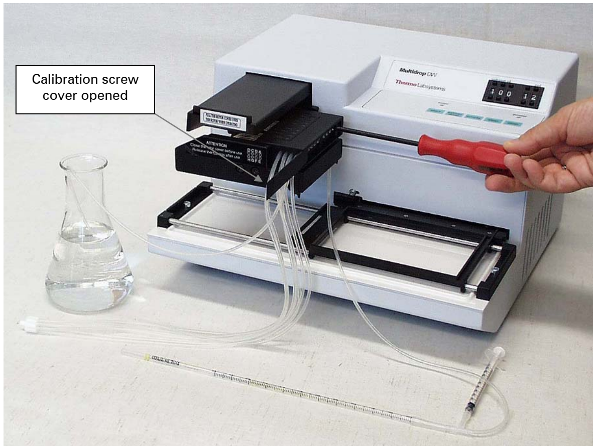
Fig. 7.7 Screwing the calibration screws according to the calibration results
